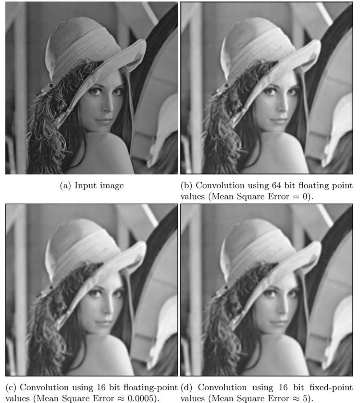
Figure 22: Convolution of an image (a) with a 5x5 Gaussian kernel. Two iterations were performed. 64 bit floating-point (b), 16 bit floating-point (c), or 16 bit fixed-point was used as underlying data type to store values. Data types with lower accuracy have only minor impact on the quality but less data has to be transferred between memory and execution units, therefore energy consumption as well as execution time is reduced. Image: Playboy Enterprises, Inc.
