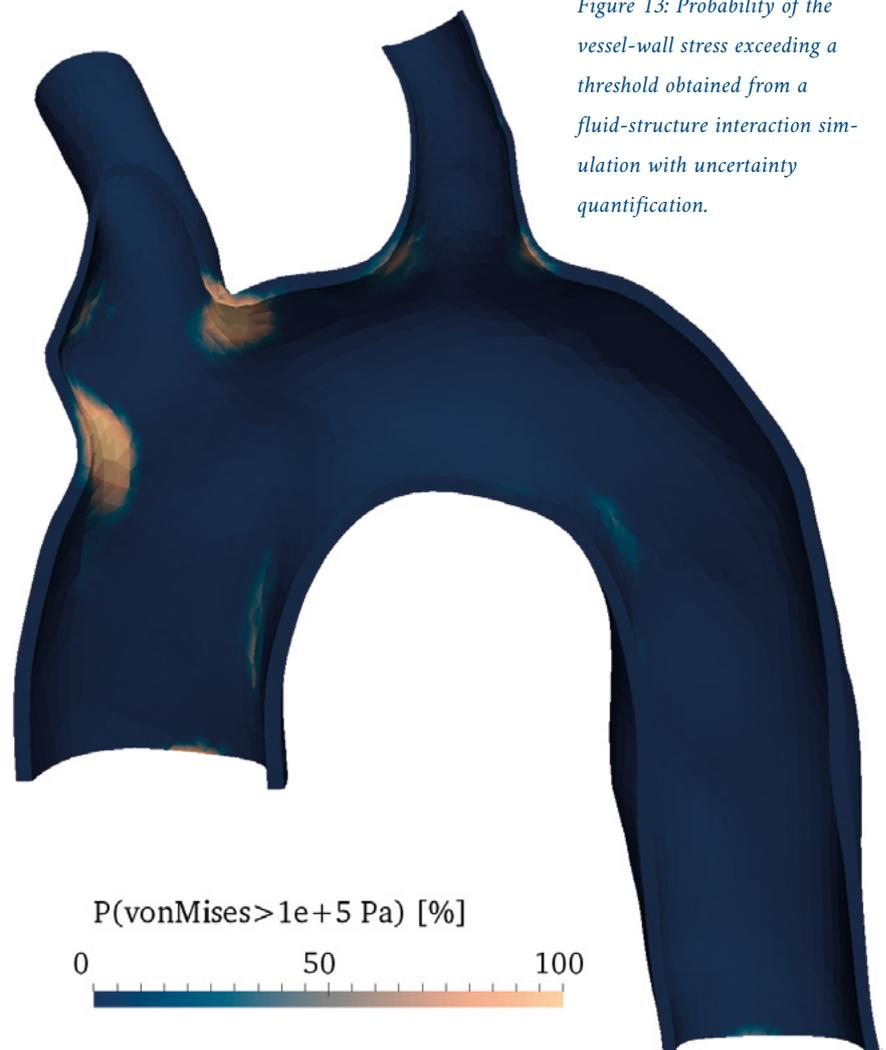
Figure 13: Probability of the vessel-wall stress exceeding a threshold obtained from a fluid-structure interaction simulation with uncertainty quantification.
