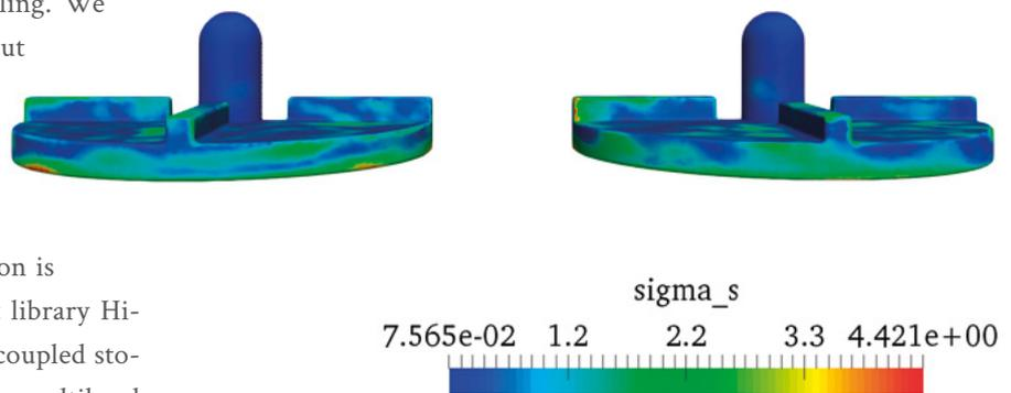
Figure 12: Standard deviation of pressure in blood pump.
