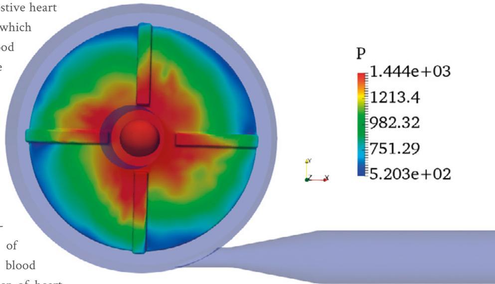
Figure 11: Mean value of pressure in blood pump.
