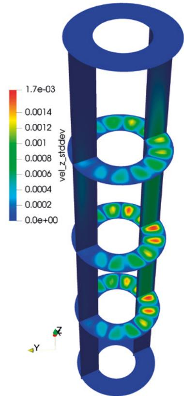
*Figure 15: Standard deviation of fluid velocity field in vertical cylinder annulus, under influence of uncertain temperature difference between inner and outer wall.*
